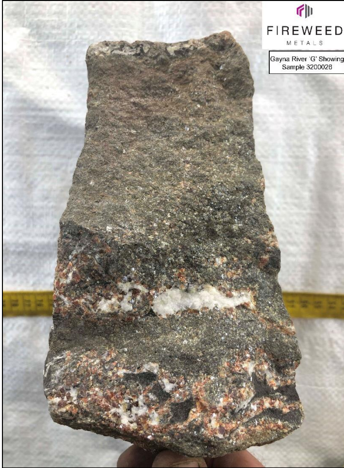
Figure 7: Gayna River 'G' showing, sample 3200026. Lower-Host angular dolostone breccia. Matrix infilled with dolomite, disseminated crystalline yellow and red sphalerite, and pyrite.
