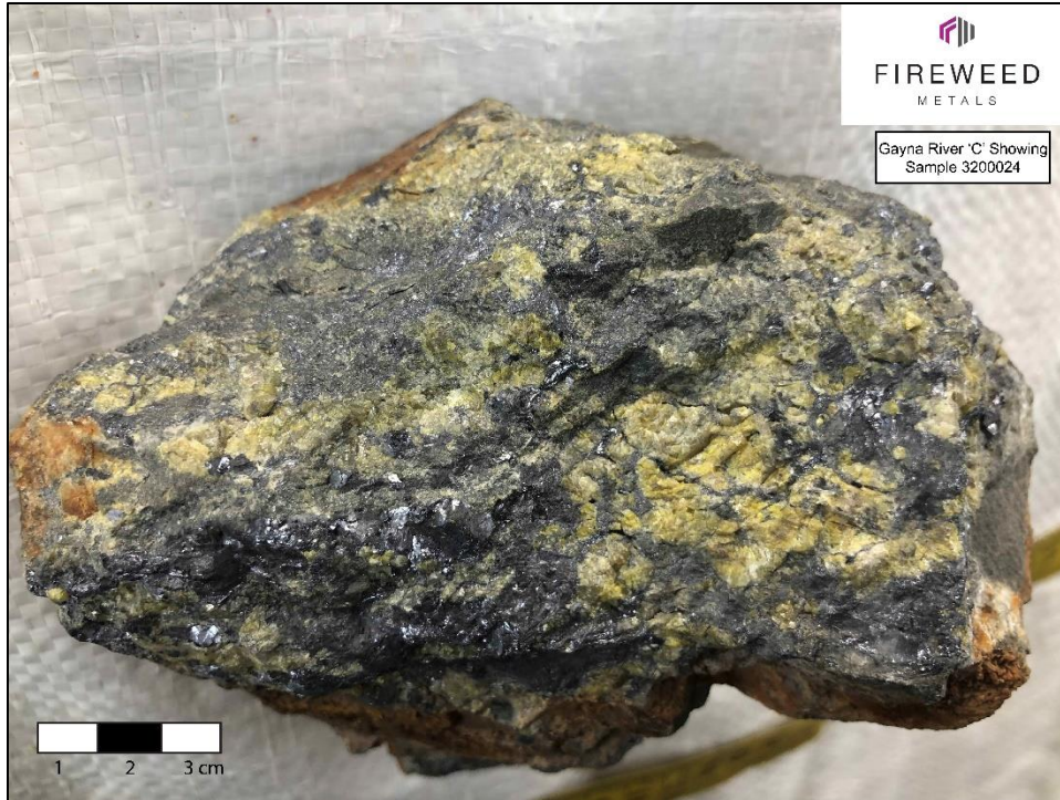
Figure 6: Gayna River 'C' showing, sample 3200024. Upper-Host massive metallic grey galena and yellow-green sphalerite.
