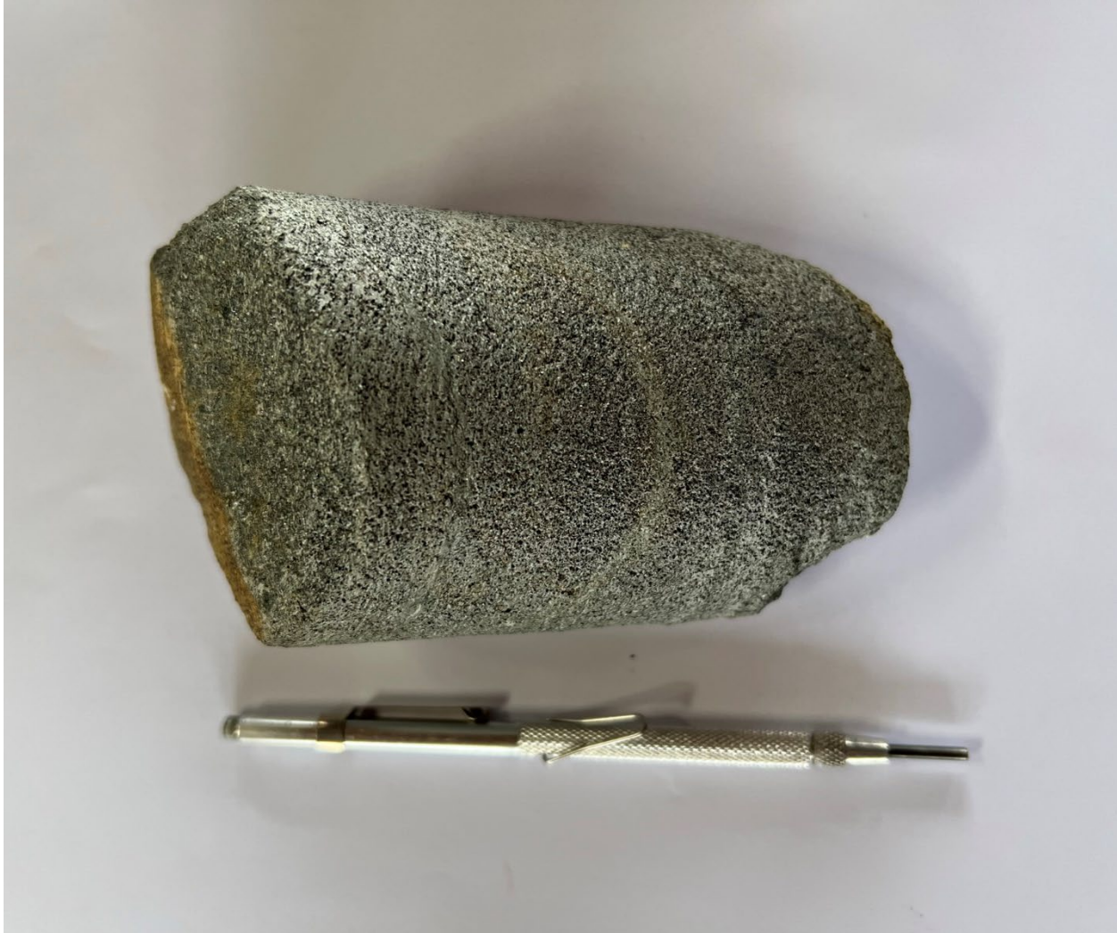
Figure 5: Photograph from a massive chromitite “core” augered from 1 to 1.2 m depth at AD22IP61A in the SW Zone of Ipueiras Target. Sample returned 2.58 g/t 2PGE+Au over 0.50 m.
