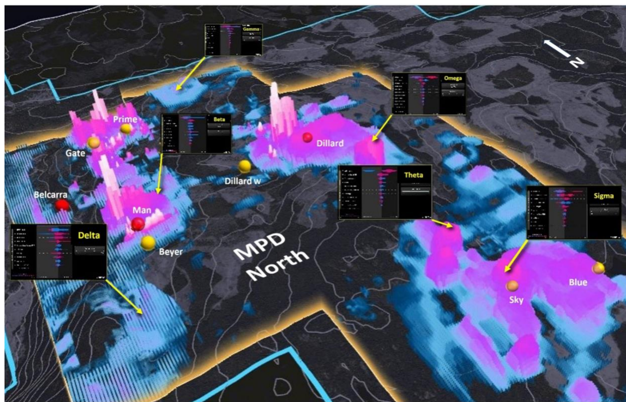
Figure 1: Screenshot of VRIFY AI 3D geo-targeting model at MPD North area. Peaks and colour contours rank predictive areas for Cu-Au-Mo mineralization. In addition to identifying known targets (spheres with white text) VRIFY AI modelling selected new prospective areas that will be followed-up in 2024 (black boxes with yellow text and arrows)
