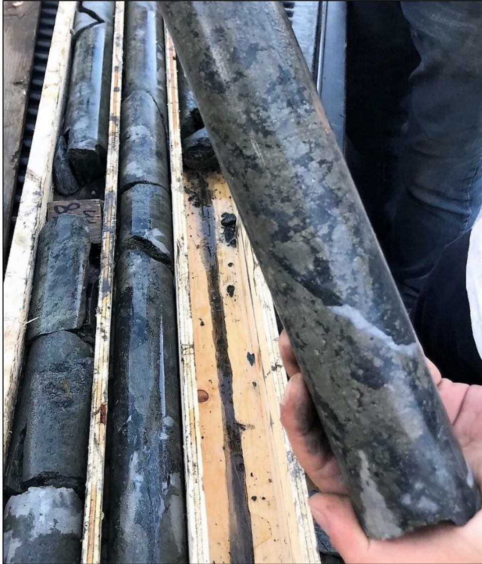
Figure 4: Example of core from 2023 drilling at the West Zone, hole AXE-23-003. New copper-gold-silver zone with semi-massive pyrite-chalcopyrite mineralization in phyllic/propylitic altered andesite breccia east of historic drilling. Core is within a 16-metre intercept reporting 0.93% Cu, 0.64 g/t Au and 3.20 g/t Ag from 274 to 290 metres.
