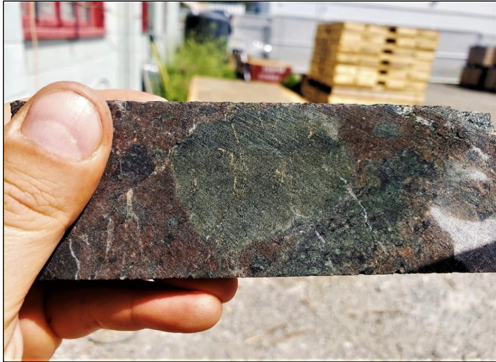
Figure 5: Two examples of core from 2023 drilling at the new lower zone, West Zone, hole AXE-23-002. Fragmental polymict breccia including chalcopyrite mineralized clasts in a potassic altered rock flour matrix with disseminated to blebby chalcopyrite and pyrite mineralization. Core is within a 30-metre intercept reporting 0.29% Cu, 0.22 g/t Au and 0.76 g/t Ag from 767 to 797 metres, towards the bottom of the drill hole.
