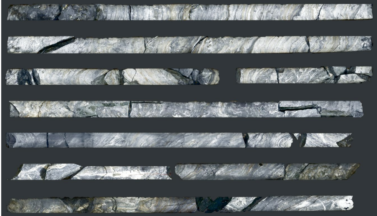
Image 1: HQ3 Core from Tom West in TS22-003, 101.0 m to 108.6 m, including an intersection 104.75-108.30 m that graded 8.3% zinc, 23.8% lead, and 396.0 g/t silver within laminated galena-sphalerite-barite (Tables 1 and 2). Image is a high resolution photomosaic from core scanning with core boxes and blocks filtered out.
