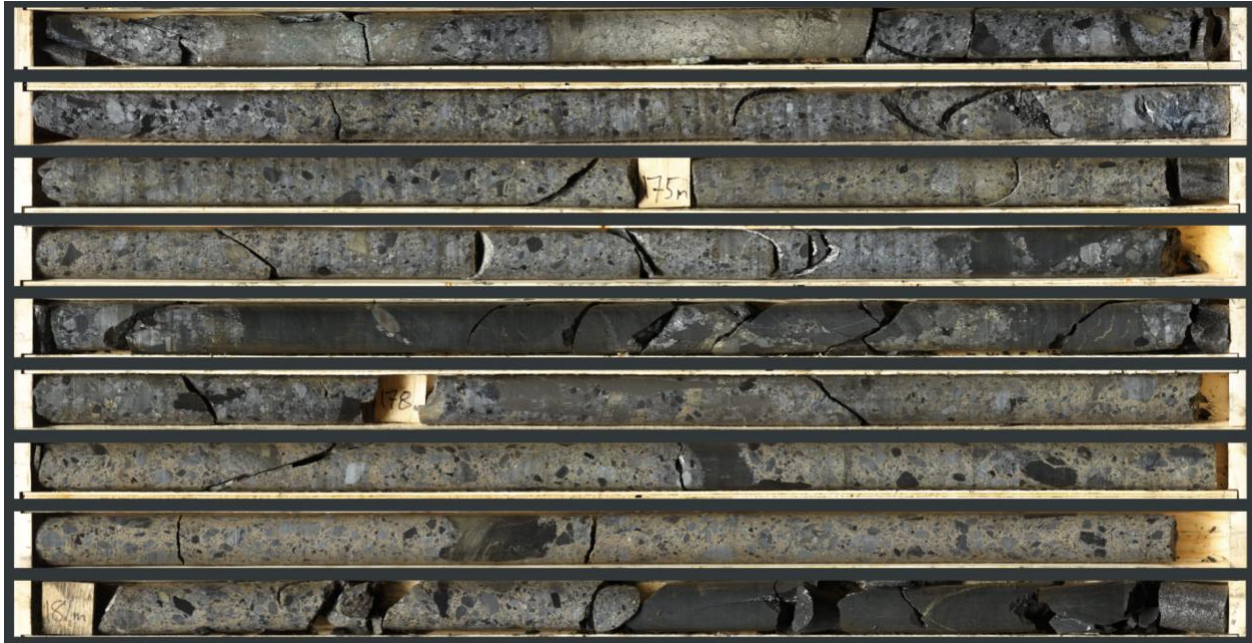
Photo 2: High resolution core scanning image of sphalerite-pyrite-siderite vein and matrix replacement mineralization in NB23-016 (172.1 m to 182.0 m).
