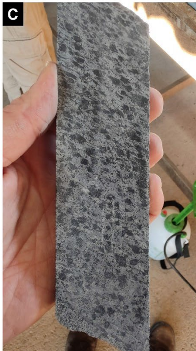
Figure 6: Salvador target. A: Drill hole DD23MES03 in progress, following up trench TR23MES02, in perspective view, looking East. B, C and D showing chromite-rich peridotites and a cm-scale chromitite reef intercepted to date in Salvador drill holes.
