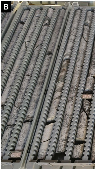
Figure 6: Salvador target. A: Drill hole DD23MES03 in progress, following up trench TR23MES02, in perspective view, looking East. B, C and D showing chromite-rich peridotites and a cm-scale chromitite reef intercepted to date in Salvador drill holes.
