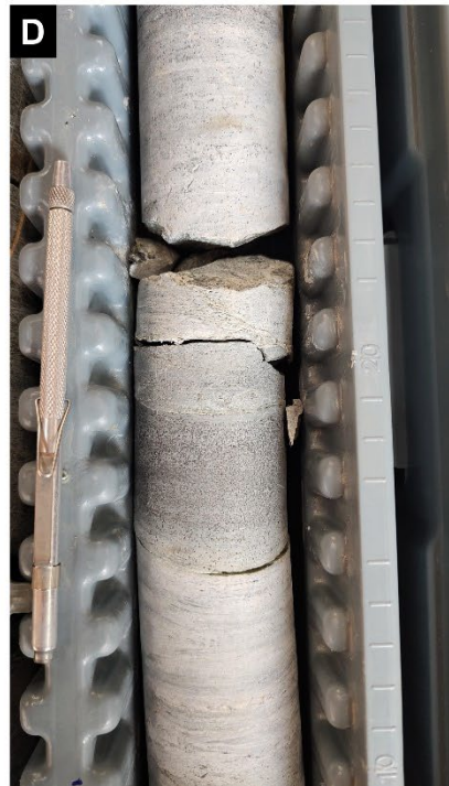
Figure 6: Salvador target. A: Drill hole DD23MES03 in progress, following up trench TR23MES02, in perspective view, looking East. B, C and D showing chromite-rich peridotites and a cm-scale chromitite reef intercepted to date in Salvador drill holes.
