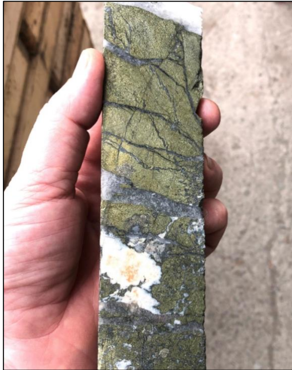
Figure 5: Example of core from MPD-23-001 at 511 m. Chalcopyrite and bornite within gypsum veins and potassic altered breccia in 75 m assaying 0.25% Cu, 0.23 g/t Au and 0.70 g/t Ag from 491 to 566 m.
